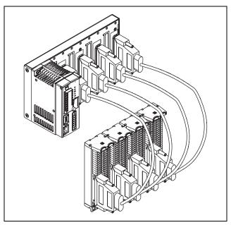
$\textbf{Figure 5.} \ \ \textbf{Compact Field Point System with DIN Rail-Mounted Terminal Blocks}$
